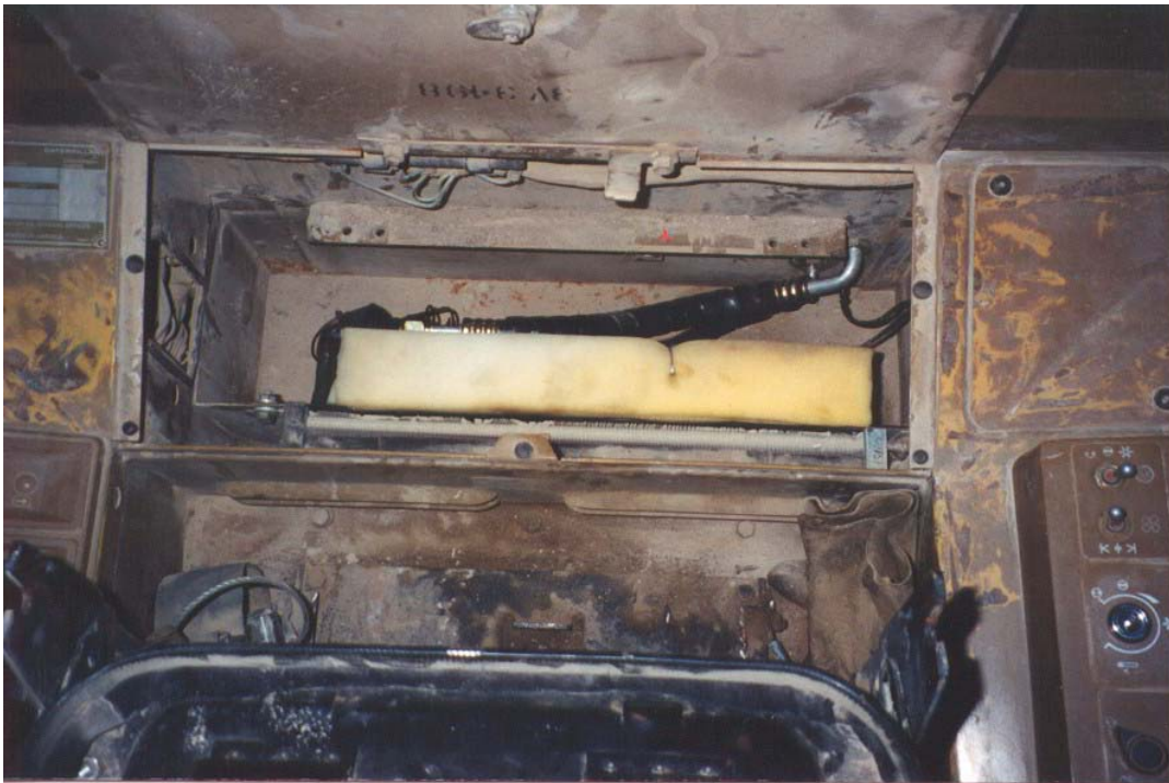
Evaporator in place for 950E, F with hoses.
